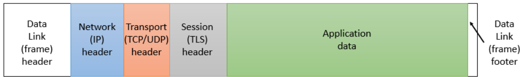
Figure 2.9: The structure of a standard Internet packet
