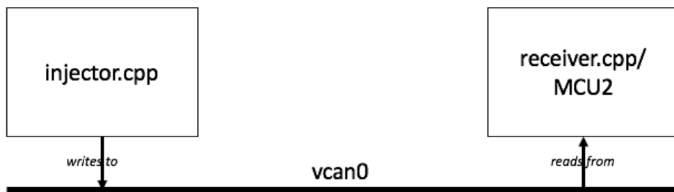
Figure 4.3: Appropriate layout of the CAN bus network for fuzzing testing
